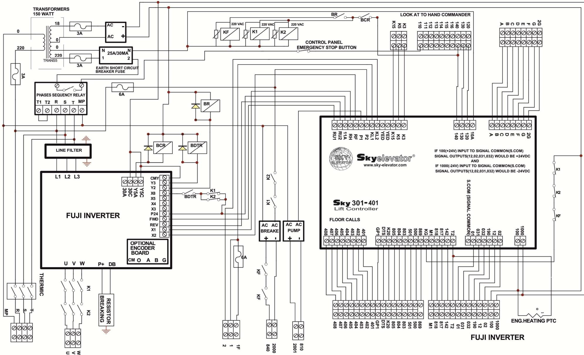
**SAFETY CIRCUIT AND CONTACTOR 220 VAC**
